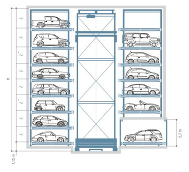
The location of the transfer room can be defined on any level within the parking levels.
