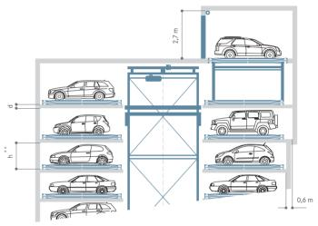
Using the option of a lateral car lift allows for transfer room location above the parking system.
