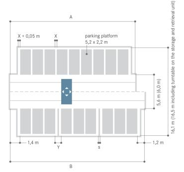
In a free standing rack structure the pallet distance  ${\bf x}$  or  ${\bf Y}$  are depending on the system height:
