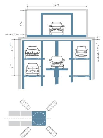
In structures outfitted with a turntable, vehicles may enter and exit at any angle position.
