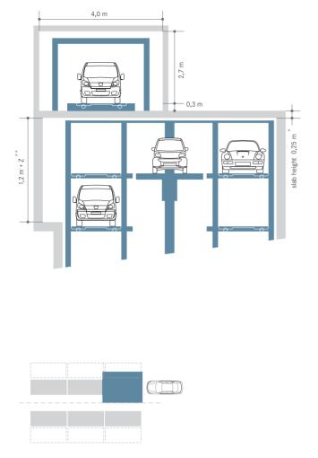
In structures without a turntable, vehicles enter and exit parallel to the rack structure.
