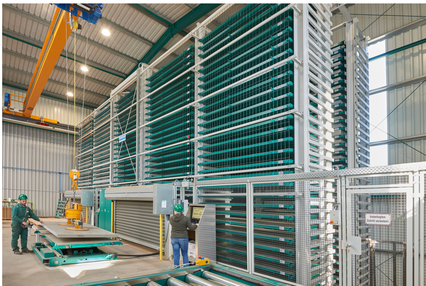
The STOPA WMS 4.0 of the automatic storage system communicates with the higher-level ERP system and with the sawing systems to be supplied
