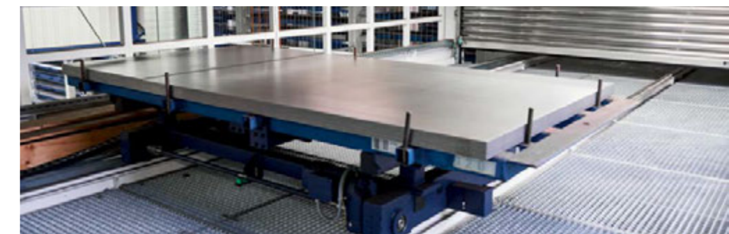
All the laser cutting machines can be supplied with material at any time from either storage system via the bridge-type passageway.
