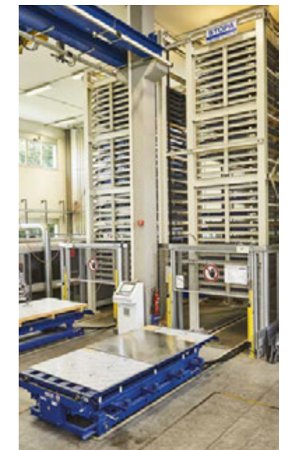
The solution with two transport carts performing simultaneous storage and removal activities makes Büchel even more versatile.
