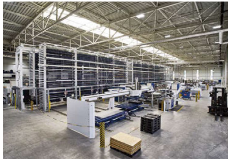
At BINDER, the STOPA COMPACT II sheet metal store acts as the internal logistics centre.
