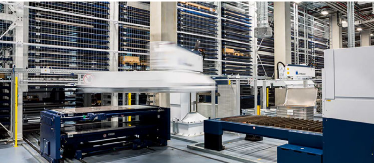
Aesculap has invested in an automatic sheet metal storage system with a modified warehouse management system.
