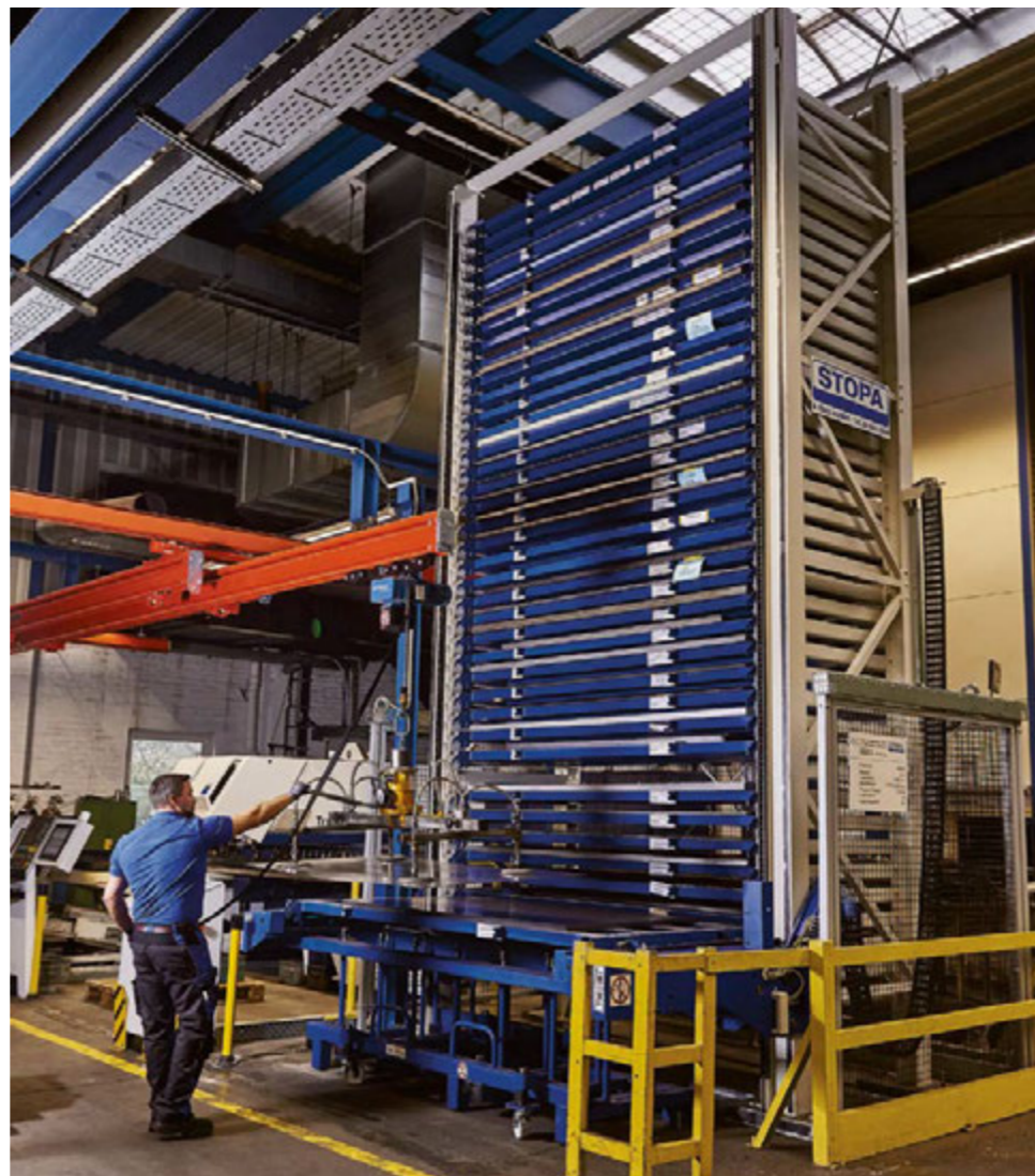
The operator makes the system pallet exit the tower and then lifts the metal panels ergonomically using the crane.
