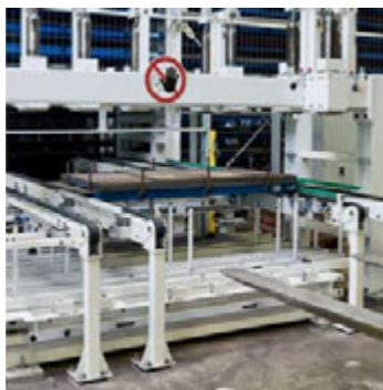
One highlight of the STOPA UNIVERSAL large-scale store installed at Dreeskornfeld is its incoming goods station which makes it possible to store all four sheet formats.
