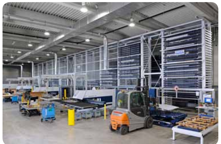
The forklift truck places the sheet stack on the deposition plungers of the incoming goods station. The sheet stack can thus be positioned without being damaged and the fork attachment withdrawn again very easily.
