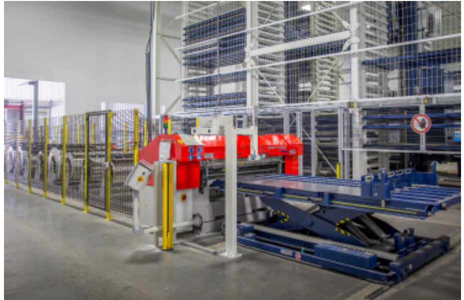
A cutting facility cuts the thin sheets supplied in coils to size, and pushes the sheets onto a flat pallet for return by a scissor lift table to the STOPA COMPACT automatic storage system.
