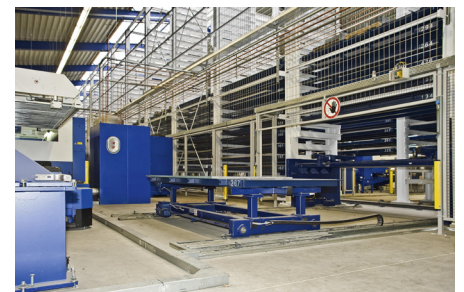
At this station, the handling component always picks up the material and sets it down in the same position. STOPA therefore installed double cars that move one above the other for storage and retrieval, saving space
