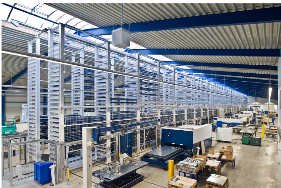
The STOPA UNIVERSAL storage system, which is integrated into Schickling's production facility, supplies material to all of the operator's laser-cutting and stamping equipment with perfect timing.
