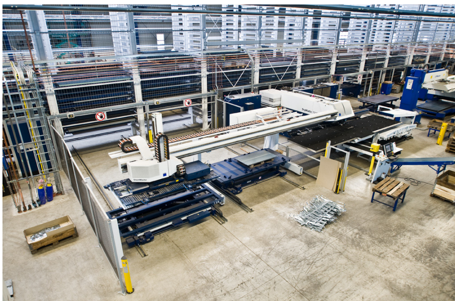
At this station, owing to the larger working area of the handling component, Schickling uses loading and unloading cars that move in parallel.
