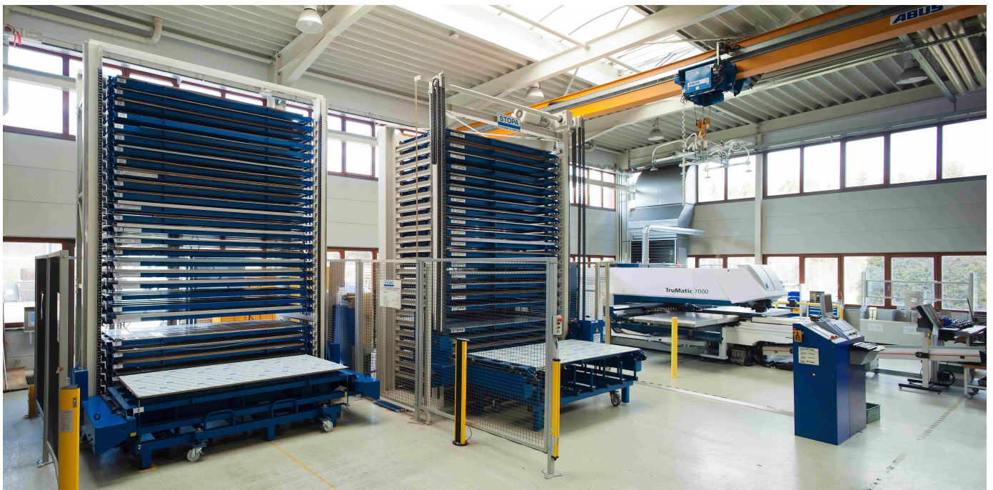
The STOPA TOWER sheet metal storage systems take up little space and are connected to the SCHAEFER laser-cutting and stamping equipment
