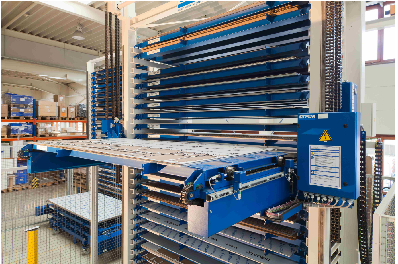
Both storage towers have a robust, low-maintenance twin-mast lifting beam that stores and retrieves items with a push/pull device
