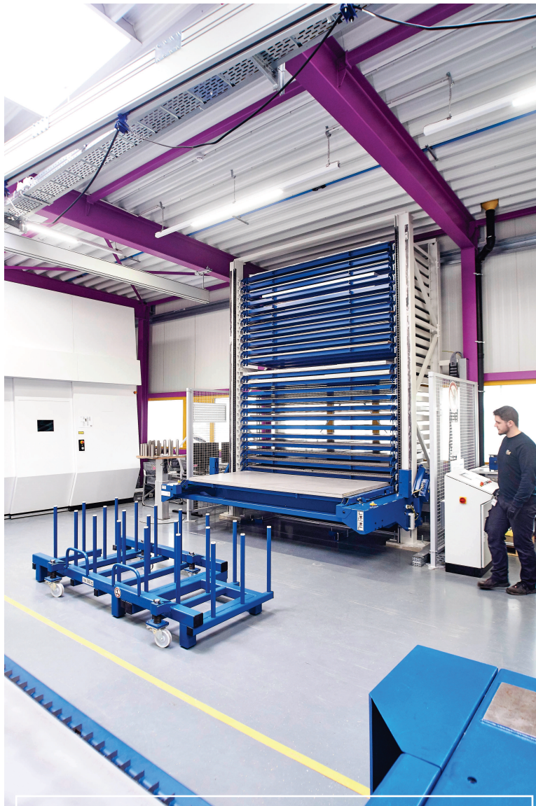
Axel Ausländer lets a system pallet pre-drive by typing the start and finish coordinates at the central control panel
