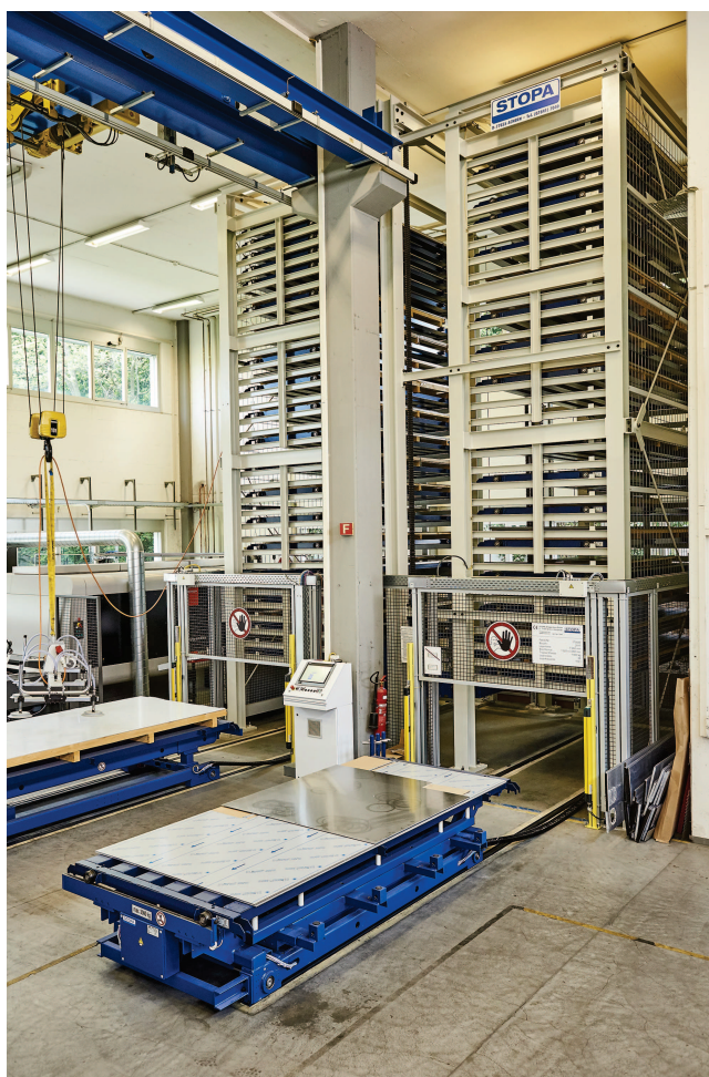
The solution with two transport carts performing simultaneous storage and removal activities makes Büchel even more versatile.
