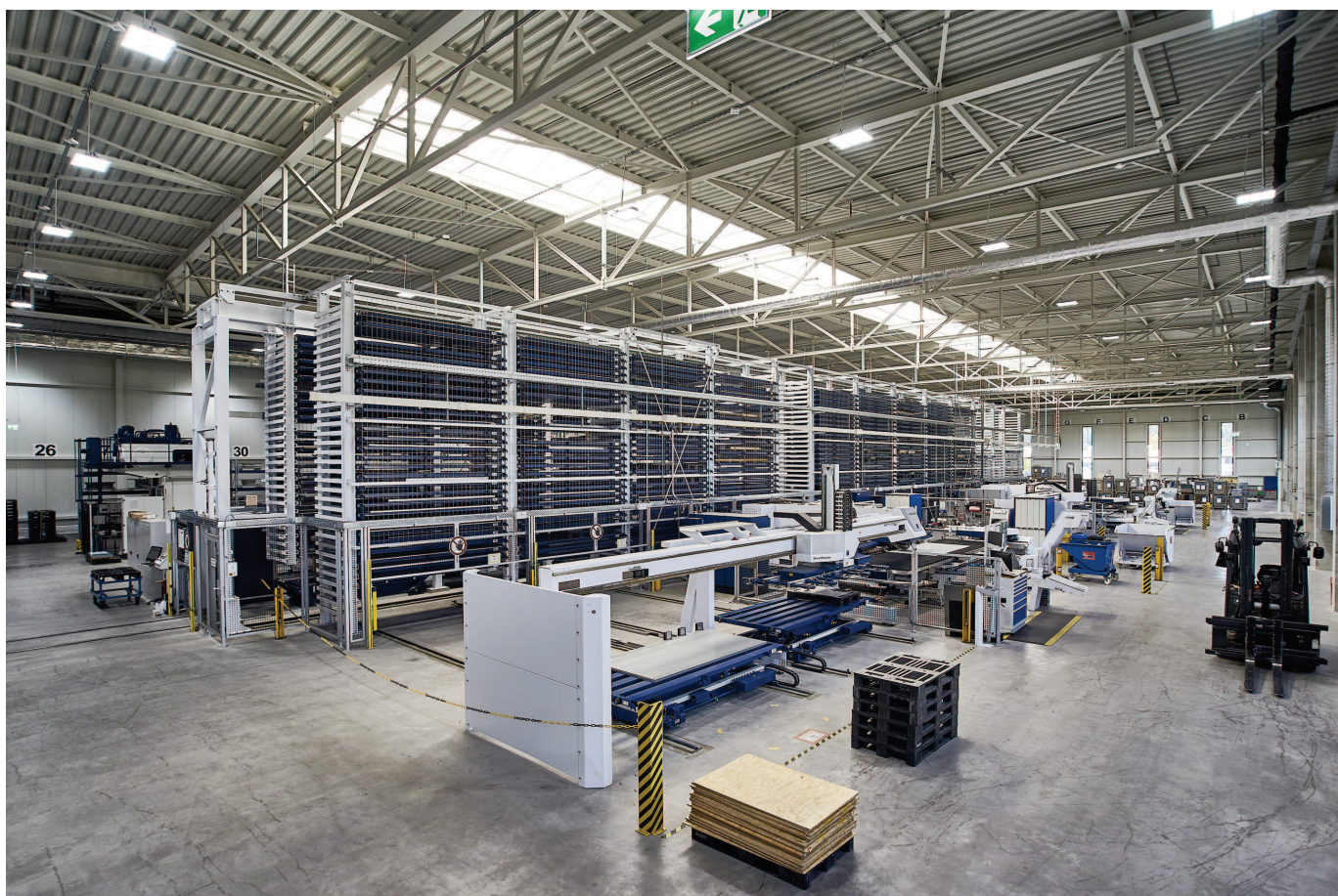
At BINDER, the STOPA COMPACT II sheet metal store acts as the internal logistics centre
