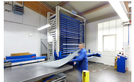
The tower storage system is right next to the stamping machine, making handling very easy.
