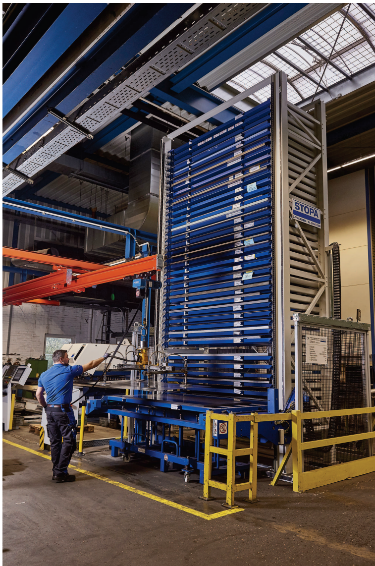
The operator makes the system pallet exit the tower and then lifts the metal panels ergonomically using the crane
