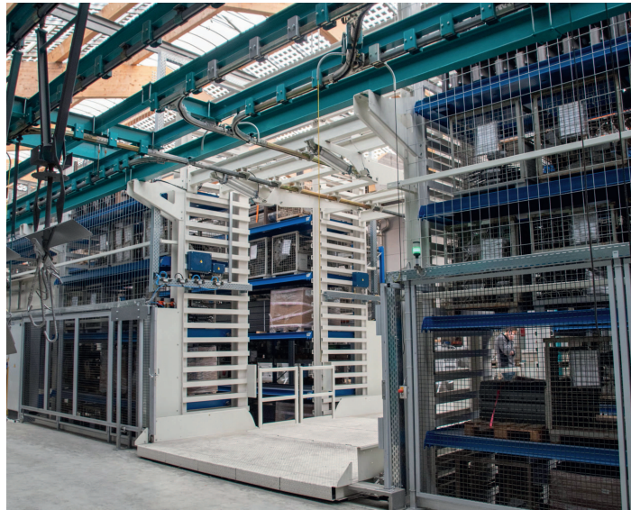
The production and assembly buildings are connected by means of a manually operated overhead conveyor system that runs through the warehouse.
