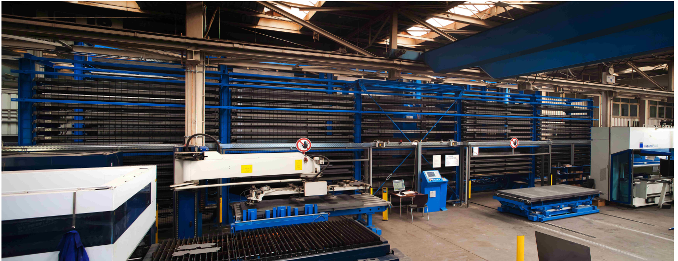
The Trumpf laser cutting system is automatically connected to the sheet metal storage system via a transport cart and a loading unit
