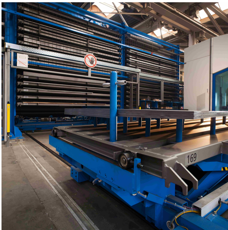
The scissor lift table lifts the stack on its plungers and lowers it onto a system pallet
