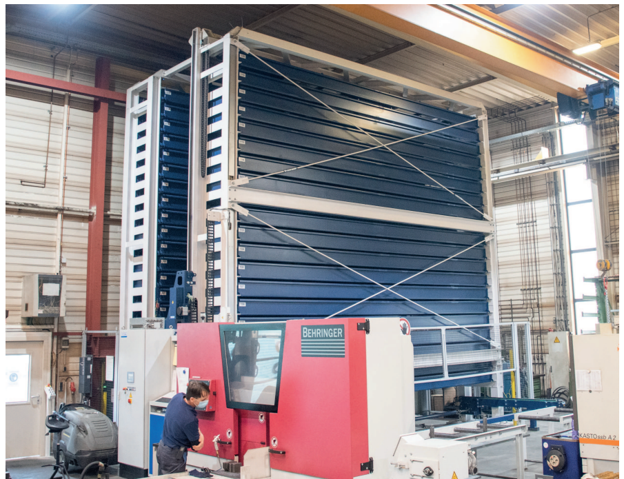
The STOPA LG-E shelving system for long-span goods saves space, increases productivity and provides quick access to material.
