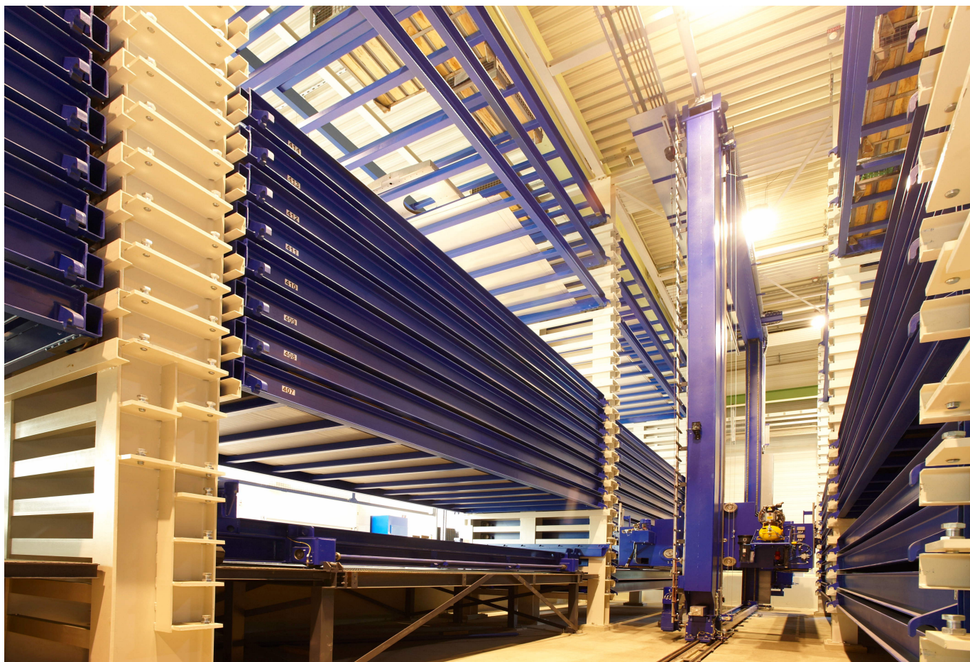
The STOPA COMPACT automatic storage system is configured here for special sheet formats up to 2,500 x 6,500 millimetres, allowing KRONES to meet its high quality standards.
