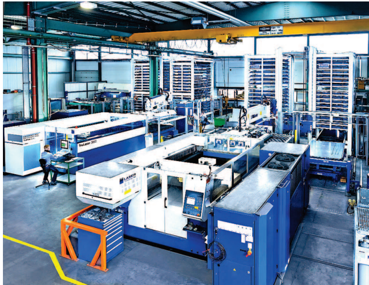
The two tower storage systems are an example of how sheet metal can be stored compactly in a relatively small area
