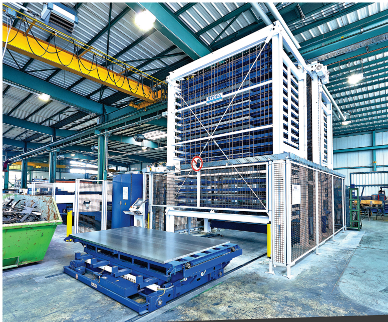
The new tower storage system has a number of important benefits: efficient use of space, fast access to sheets and short throughput times
