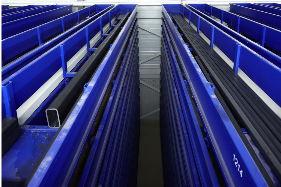
The long-span goods shelving system provided by STOPA uses space very efficiently and provides fast, random access to the material
