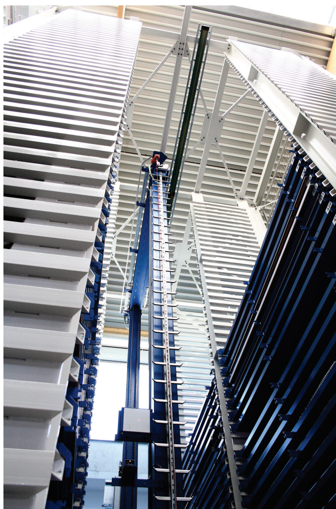
The STOPA COMPACT II sheet metal storage system links two storeys intralogistically
